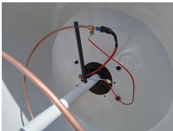
Quarter-wave stub is connected to transformer behind reflector.
