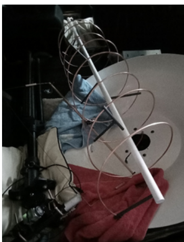
The entire antenna disassembles in five minutes and fits in an average-sized vehicle.
