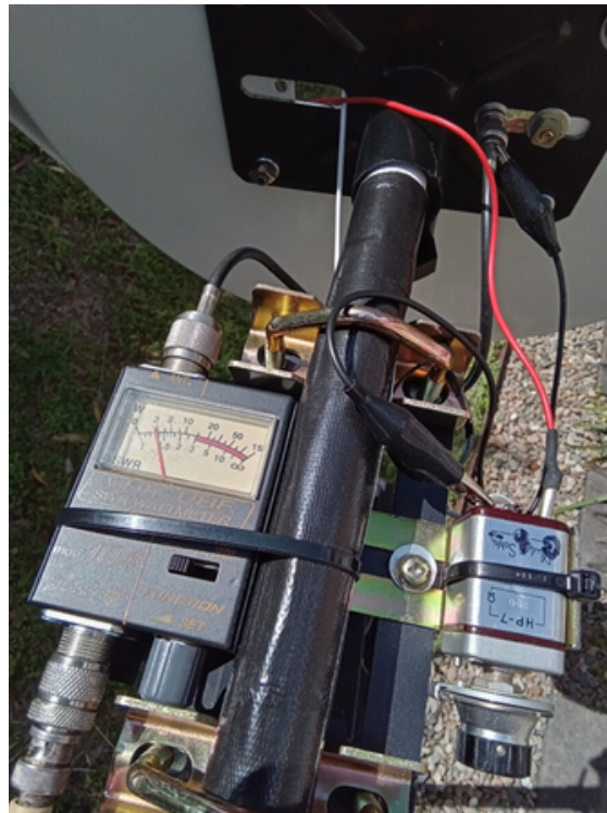
'Firing end' rig showing stub connections to impedance matcher and center dowel support in pipe, mounted to the adjustable-angle speaker-platform. This connects to the radio shelf.
